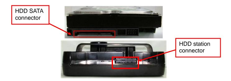
Push the hard drive towards the SATA connector and make sure the SATA connector is properly connected.
