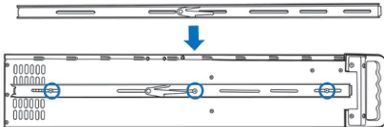
Now put the center slide right next to the rackmount chassis. You should be able to find screw holes on both slides of the chassis. Later, the center slide will be used for attaching the sliding rail.
