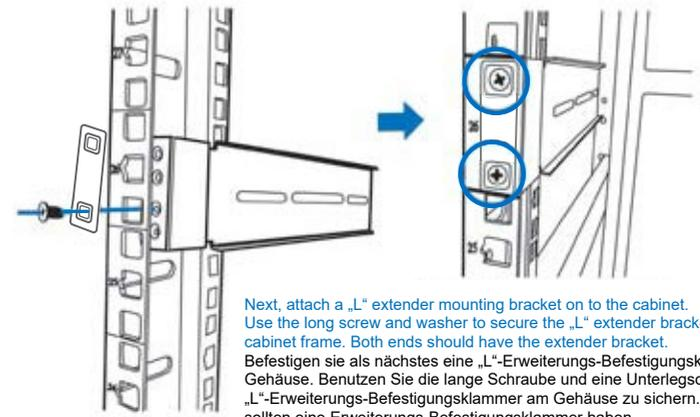
Next, attach a „L“ extender mounting bracket on to the cabinet.
