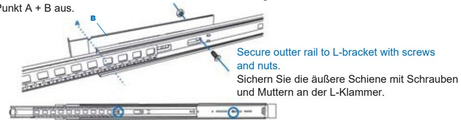
Secure outer rail to L-bracket with screws and nuts.
