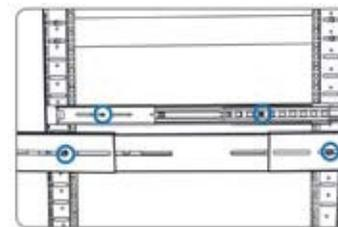
Repeat previous steps to secure sliding rails on both sides.
