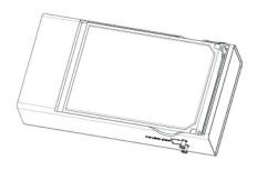
d) Put the aluminium housing back to the inner tray and then fix the housing at the bottom side by the longer screws. After this, the installation of the HDDs is done.
