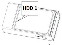
c) Fix the HDDs with the **shorter** screws at the upper side of the inner tray. You will find the print "Fix HDD here" at this position.
